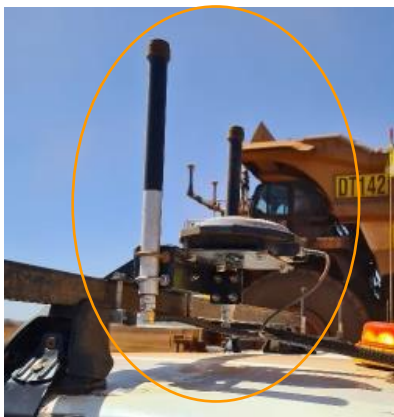
SAB V3 Antenna Station mounted to LV roof bracket
